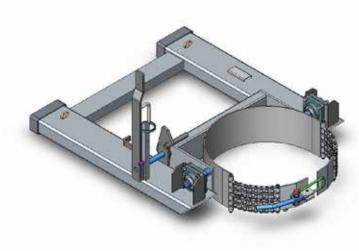
The type DC-T Cord Operated Drum Rotator is designed for fast and economical 205 litre drum emptying. A Chain Belly Strap with an eccentric lock holds the Drum firmly in position. To release the drum the Operator pulls the draw chord from the driver's seat. With the drum C of G forward of the pivot point, the drum tips forward 180°+ automatically.
