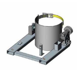
The type DR-NC Drum Rotator with the PBO Cradle fitted is designed to lift and rotate plastic Drums and Barrels as well as 205 litre steel Drums through 360° above the chest height of the Operator. A Hand Chain is used to rotate the Drum/Barrel via a Gearbox for controlled rotation. The dual Woven/Chain combination Belly Straps holds the Drum/Barrel firmly in position.
