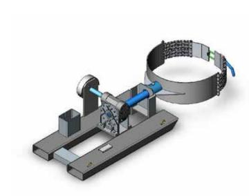
The type SW-NC Sideways Drum Rotator is designed to lift and rotate 205 litre Drums through 360° perpendicular to the fork arms. A Hand Chain is used to rotate the Drum via a Gearbox for controlled rotation. A Chain Belly Strap with an eccentric lock holds the Drum firmly in position.
