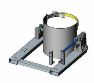
The type DR-NH Drum Rotator with the PBO Cradle fitted is designed to lift and rotate plastic Drums and Barrels as well as 205 litre steel Drums through 360°. Handle rotation of the PBO Cradle via a Gearbox, ensures minimum effort for fully controlled tipping, allowing complete emptying of the Drum/Barrel contents. The dual Woven/Chain combination Belly Straps holds the Drum/Barrel firmly in position.
