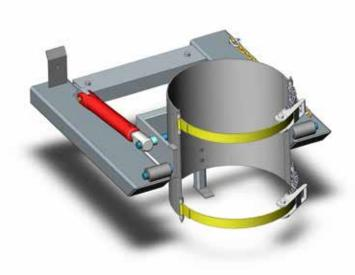
The type DCR2-PBO Hydraulic Drum Rotator is designed to lift and rotate Drums with varying diameters including standard Plastic Drums as well as barrels using dual woven/chain combination Belly Straps with ratchet tightening for clamping. Rotation is provided by the Forklift hydraulics and controlled by the 3<sup>rd</sup> function lever.
