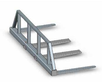
The type FS3-LG Fork Spreader & Load Guard has been designed to safely lift extra wide or flexible loads without the risk of damage to products such as plasterboard, roof sheeting, timber or plastic tubing etc. The Fork Spreader evenly distributes the load over its full length and has the extra benefit of a load guard incorporated into its design. This slip-on attachment is easily fitted onto the Lift Truck fork tines and is secured by a safety chain.
