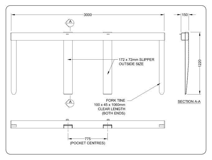
Forklift Systems Ph: 1800 688 788 or +61 2 9897 5111 sales@forkliftsystems.com.au www.forkliftsystems.com.au www.forkliftsystems.com.au
