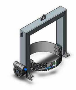
The type CDR-500H Crane Drum Rotator has been specifically designed for use by Crane. The Drum is quickly clamped into the holder via the twin Chain Belly Strap allowing 360° rotation.
