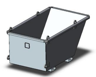
The type CB20 Crane Bin is manufactured from 5mm plate to allow transport of heavy waste such as sand, gravel, excavation waste and scrap metal.
